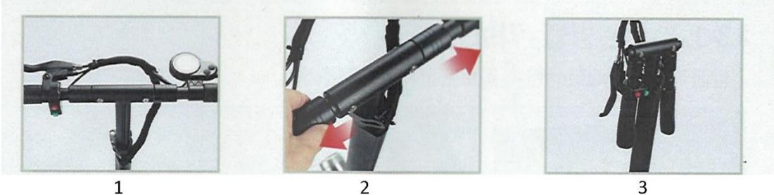
Open the quick-release clamp, push down the handlebar and lock the clamp. Pull out both sleeves to open the folding mechanism and fold the handlebar. If the sleeves move rigidly, push the handles upwards while pulling the sleeves ourwards. You can also lubricate the sleeves.
